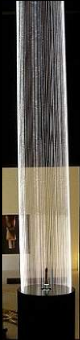
scattering optical fiber 2mm tensioned using springs. Display Estée Lauder
