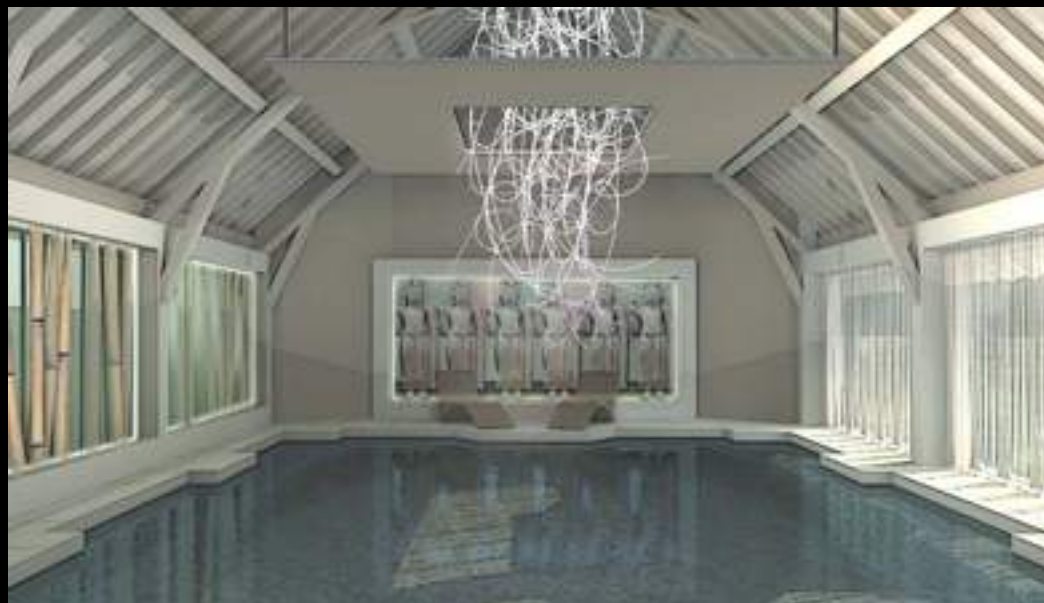
scattering optical fiber 2mm tensioned using springs. Display Estée Lauder
